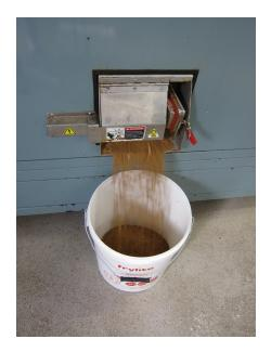
solids were stored in sealed buckets and the condensate was emptied into a sanitary sewer drain. Once the solids were placed into a storage bucket, a 200 gram sample of the product was placed into a labeled zip lock plastic bag for laboratory testing. Lastly, the electric meter was read and a note of kilowatt hours used was recorded for each batch.
