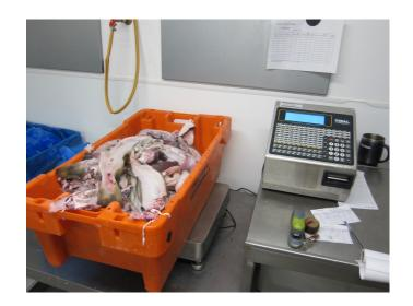
1. Weigh input materials on an electronic digital scale in 40kg batches.
