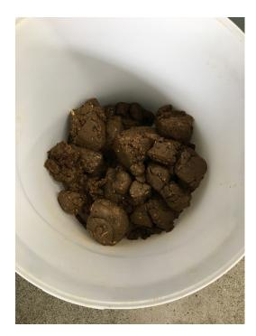
Shown above are the solid outputs from haddock processing residuals to the left and from whiting processing residuals to the right, in chunky balls.
